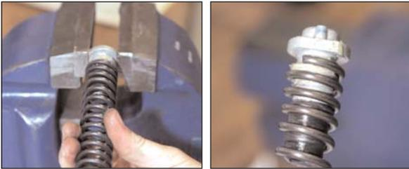
12. Put the lower part of the fork leg into the vice, and again use the channel-lock pliers to remove the stock spring, turning it clockwise, and again re-install the other end of the supplied heavy-duty spring.
