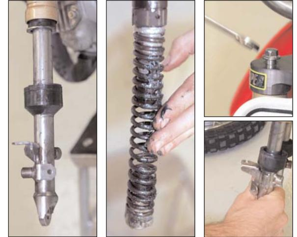
19. Next, reinstall the circlips just like you found it to begin with, and then use an open ended wrench to push it into place until it makes an audible clicking noise.
