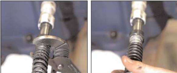
13. Put the flat, gray bushing at the bottom of the fork spring into the vice, **but be gentle with it because it can break**. Take a 1/8-inch drift and a hammer and punch out the pin as you see here. **Do not lose this pin.**
