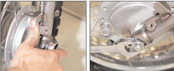
23. Re-install the fork guards using a 5mm Allen wrench.
