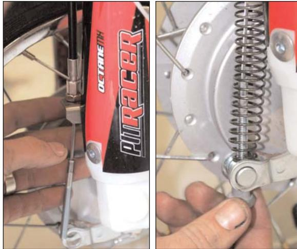
26. Adjust the brake cable to the desired tension.
