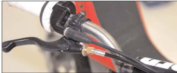
25. Route the bottom end of the brake cable through the fork guard and then through the top tab on the fork tube. Then replace the spring you removed in Step 4, route the threaded end through the tab on the brake assembly, and then replace the wingnut to hold the brake in place.
