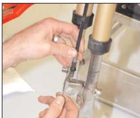
6. Remove the front-brake cable from the front-brake lever. Throw the cable in the trash.
