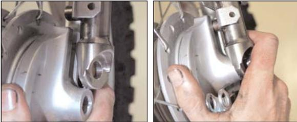
22. Now, re-install the front axle and tighten it using a 14mm wrench on the rider's right and a 19mm on the rider's left.
