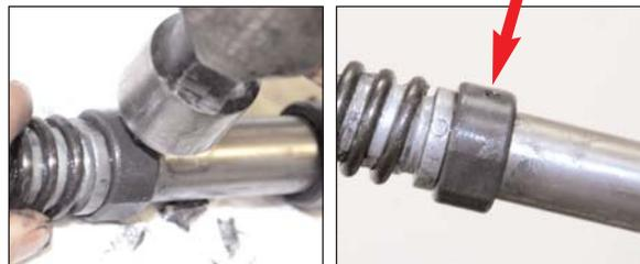
17. Keep in mind, when you put the fork internals back into the fork tubes, the notches on the top of the internals point toward each other in the front end of the bike.
