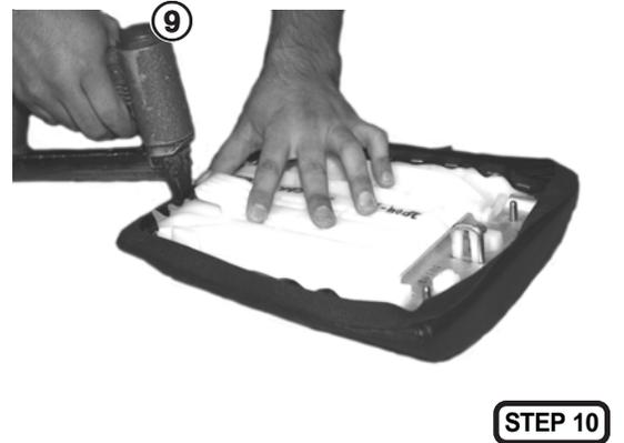
**STEP 11:** Space the staples approximately 1/2-inch apart around the perimeter of the seat base ⑩. Alternate staple installation from side-to-side and top-to-bottom.
