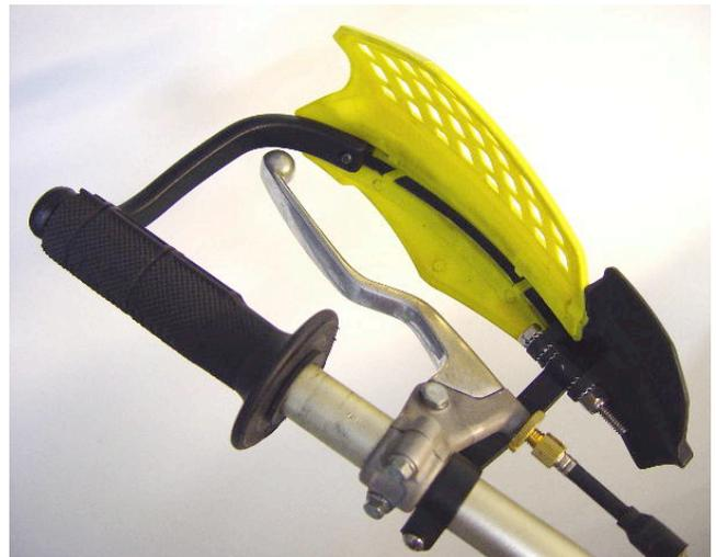
**Helpful Hint:** To remove the clamp from inside the handlebars, first loosen the flat head screw 3 - 4 turns, then tap the head of the screw to push the cone further inside so the clamp will slide out.
