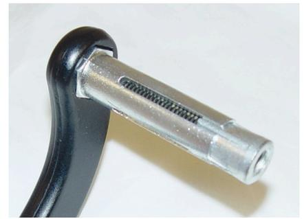
**Steel Handlebars:** Assemble the Hand Wrap clamp onto the bracket by inserting the flat head screw through the bracket, sliding on the rubber tube and threading the flange nut onto the screw (as shown in the picture). Insert the clamp assembly into the end of the handlebar and tighten the flat head screw with a 5mm hex wrench so the bracket is slightly loose.
