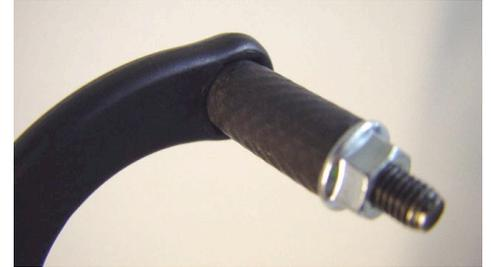
**Helpful Hint:** Apply lubricant between the flat head bolt and the bracket. This will enable you to get the hand wrap clamped tighter to the handlebars.
