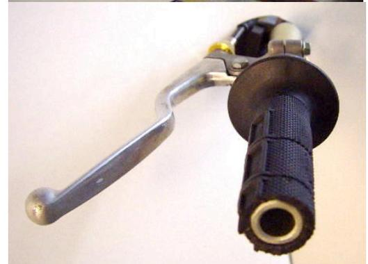
**STEP 5: Aluminum Handlebars:** Assemble the Hand Wrap clamp onto the bracket by inserting the flat head screw through the bracket and threading into the cone (as shown in picture). Insert the clamp assembly into the end of the handlebar and tighten the flat head screw with a 5mm hex wrench so the bracket is slightly loose.
