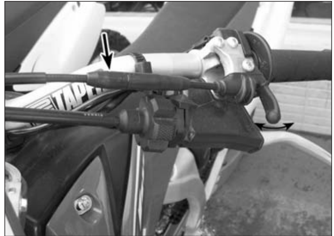
5.14a Measure freeplay of the hot start lever at the lever tip - slide back the cover (arrow) for access to the adjuster . . .
