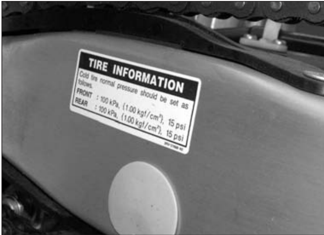
2.1 Decals on the motorcycle include maintenance and safety information
