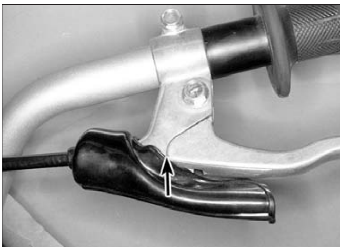
6.1 On some models, clutch freeplay is measured at the lever gap (see this Chapter's Specifications) . . .
