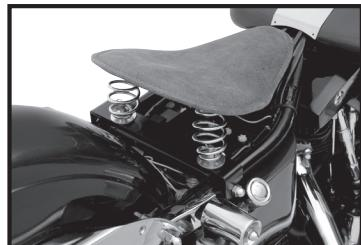
11. Install your seat holding the back up off the studs while installing the 3/8" hinge bolt. With the hinge bolt in place, flex the springs to align and slip over the lower mount studs.
