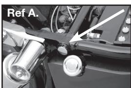
3. Remove the two hair pins, acorn nuts, lock washers, 3/8" threaded rod and the aluminum step spacers from the mount assembly. Ref B.
