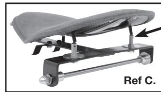
10. Install rear seat springs at this time. Turn your seat over and lay on a soft surface. Install fender washer, spring, flat washer, lock washer and hex nut onto rear seat studs.
