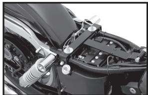
6. With the front bracket on the seat mount loose, slide bracket forward making sure the fingers of the bracket are secure under the frame. Tighten the two 1/4" button head screws at this time. No up or down movement should be present after installation.
