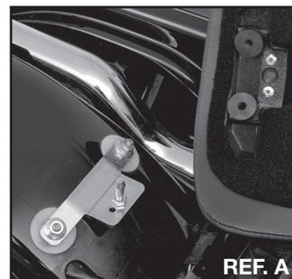
7. The stud and the Jam nut should be loose in the bracket at this time. Adjust the receiver stud so there are approximately three threads out of the bottom; see REF. B. This will be a good starting point.
