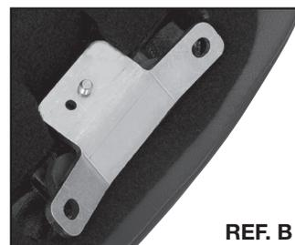
**NOTE:** On 2008 models, the stud should be flush to the bottom of the bracket. For final adjustments, in some cases it may be necessary to add a washer-spacer between the fender and mount bracket to obtain the proper height.
