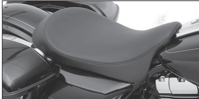
2. Remove rear mount screw; remove seat. The rear Phillips-head screw will not be reused for the solo front installation.
